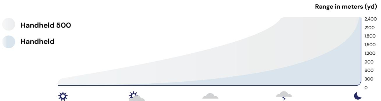
The Handheld comes in two models with different laser output power: Agrilaser Handheld and Handheld 500. Choosing the right model is essential in order to generate a laser projection with sufficient contrast for effective bird dispersal.
